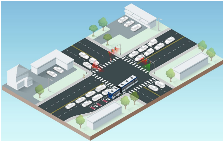
Figure 10: Bus bypass/approach lane with queue jump signal
