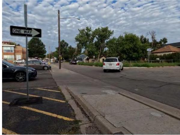
Figure 28: The exiting driveway of the parking lot does not have many amenities that support drivers or pedestrians. Students use the sidewalk to enter the school, but parked cars sometimes extend into the sidewalk, reducing the total walkable width. Cars parked along the street limit sight visibility.
