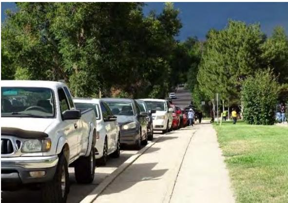
Figure 29: A queuing car line on Depew Street where 1st and 2nd graders are dismissed after school. As a one-way street, pedestrians will only need to be concerned about approaching vehicles from the southbound direction. Cars are parked on both sides of Depew Street which causes congestion and reduces the space drivers can maneuver. Students are crossing the street at all locations to get to their vehicle.
